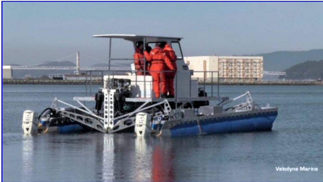
The Velodyne Martini 1.5 at rest, with its suspension lowered. The boat pilot can manually adjust the suspension and the height of the boat deck.
