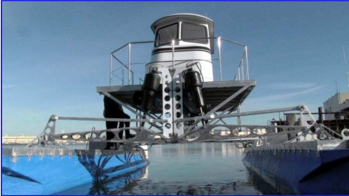
A view of the Martini 1.5 shows the front suspension legs and the airbag and actuator components.
